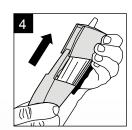
Slide the cover into the grooves until the lower end snaps into place.
